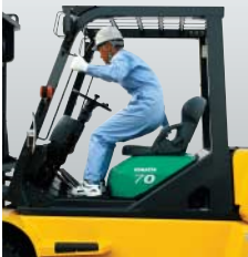
When the operator leaves the seat, OPS is activated
