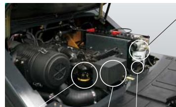
Fuel main filter Relay and fuse boxes are arranged in the same location
