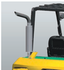
Upward exhaust muffler
